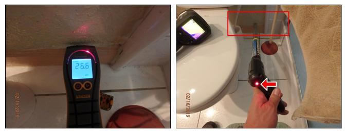
**4.8** Area(s) of previous water intrusion/staining. The area(s) were scanned with an infrared thermal camera and checked with a moisture meter and found non-resultant for active moisture at the time of the inspection. These areas should be painted.
