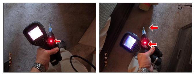
**4.7** (2) There are elevated moisture levels (moisture content above 17%) at the wall behind a toilet. Unknown reason as to why or the moisture content is elevated. This area should be monitored.
