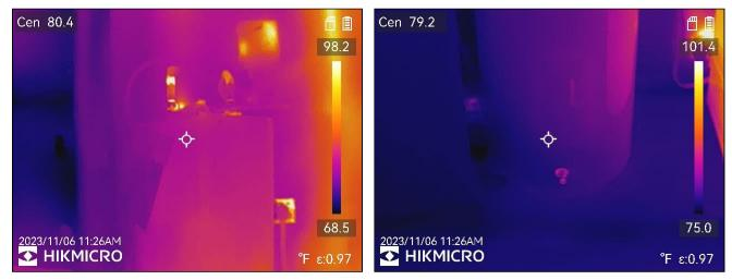
**7.5** (1) One or more areas of active leaks noted. The leak could be from the drain or the supply lines. All leaks should be addressed expeditiously in order to avoid moisture damage and mold growth.
