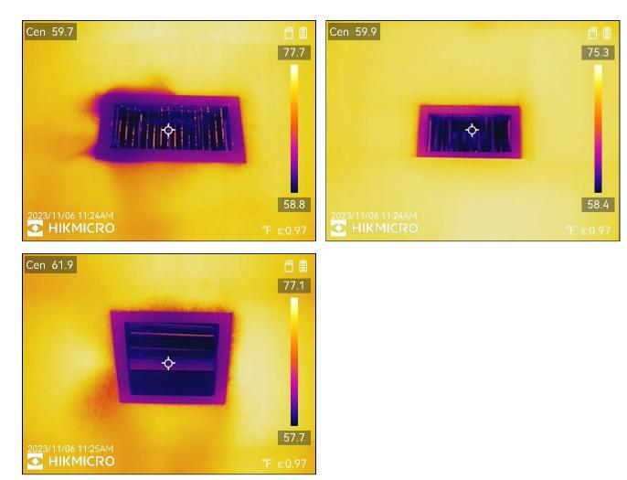
**8.3** The HVAC system did NOT produce heat using the installed operating controls. The thermostat was set to HEAT and the setting was raised to the upper limit in order to call for heat. After a few minutes the heat was not adequate. It is possible that there is no heat kit installed. Recommend further evaluation by a qualified HVAC contractor.
