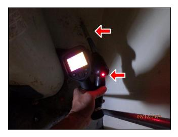
**4.7** (2) Both buildings: There are multiple areas along the baseboard which have elevated moisture levels. The moisture sensor triggers at 17% which is considered elevated for drywall. The reason for the elevated levels is not known.
